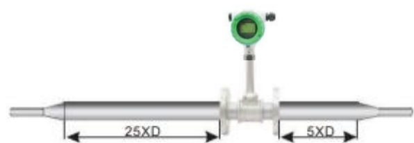
Concentric Expansion Pipeline
