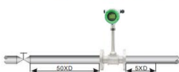
Regulating Valve, Half-open Gate Valve
